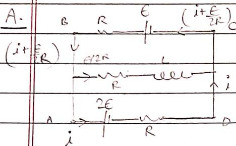
Initially  $i = \frac{E}{2R}$  flowing through ind. (steady state)
