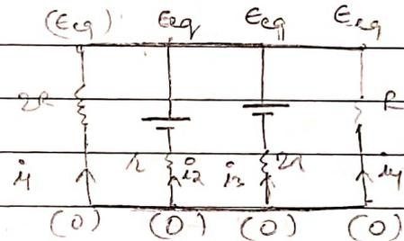
$i_1 = \frac{Bvl}{2(\lambda r)}$       $i_2 = \frac{\frac{BvlR}{\lambda r} - Bvl}{\lambda} = -\left( \frac{Bvl}{\lambda r} \right)$       $i_3 = \frac{-Bvl}{2(\lambda r)}$       $i_4 = \frac{Bvl}{(\lambda r)}$
