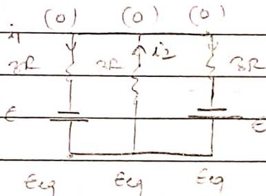
\* We can represent induced emf with a battery anywhere in circuit except the common side
