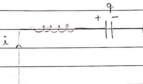
$\Rightarrow V_C = \frac{q}{C} \Rightarrow \frac{dq}{dt} = -\frac{q}{LC} \Rightarrow$  current starts flowing in opp. direction
