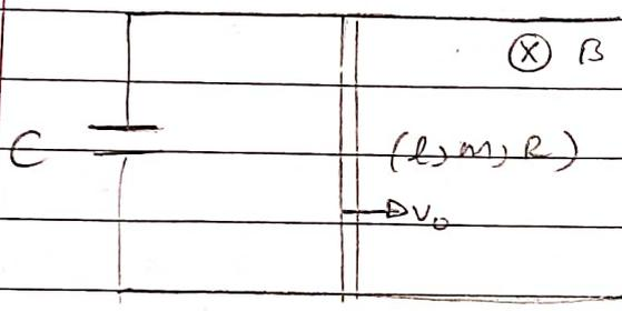
Find charge on cap., current in circuit & force req. to move rod with const. vel. as a f<sup>n</sup> of time.
