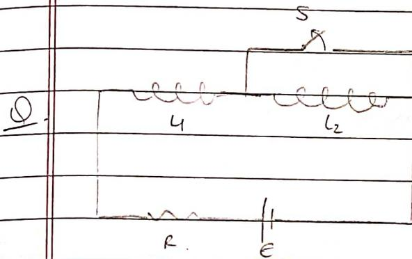
Find current immediately after opening S. & in new steady state
