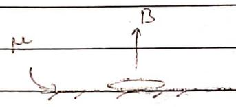
At  $t=0$ , a vertical B co-axial with conducting disc is switched on
